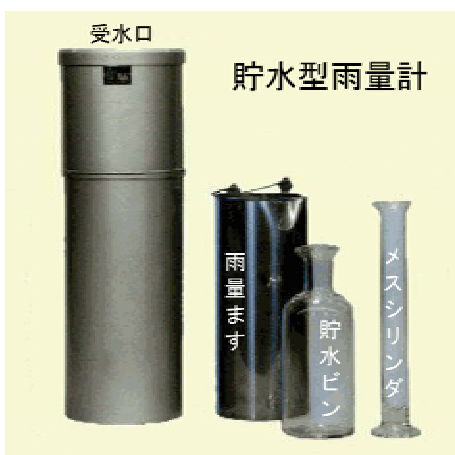
Figure 2.18 Examples of simple daily rain gauges
