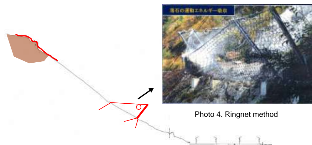
Figure 4. Longitudinal profile of the slope and the application of the ringnet method
