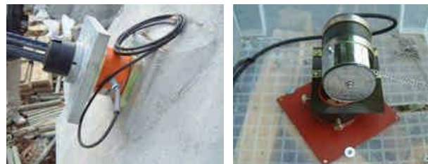
Photo-1 Anchor load meter (left) and tension meter using strain gauges (right)
