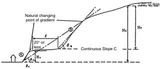
(b) When the viewing angle is  $30^{\circ}$  or more ( $\theta_c \ge 30^{\circ}$ )
