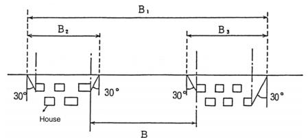
B > 50 m: The hazard area shall be handled as 2 places called B<sub>2</sub> and B<sub>3</sub>.
