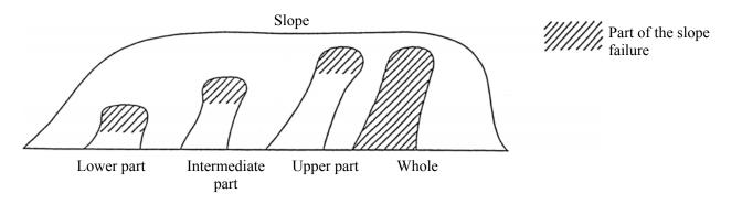
Fig-19 Position of an occurrence of a failure
