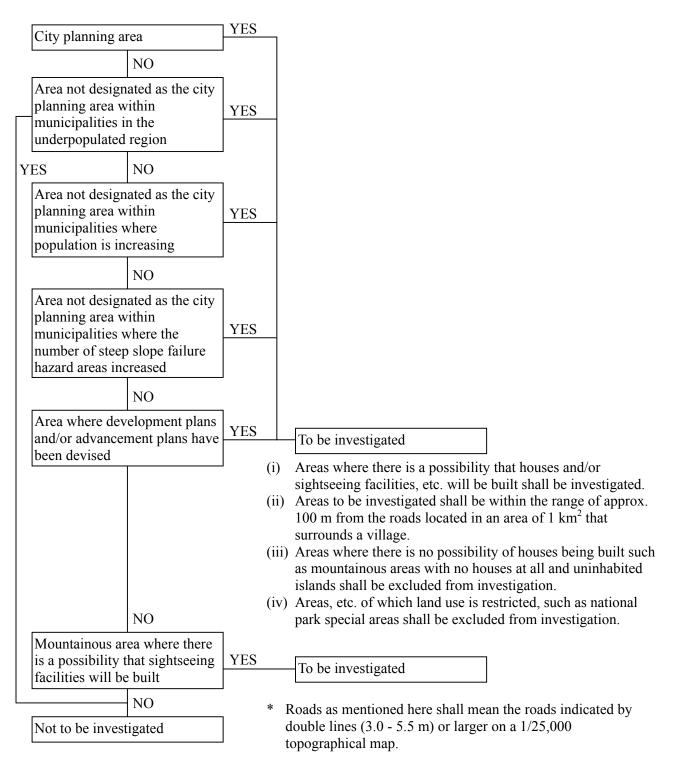
Fig-3 Image of the selection of the range to be investigated on a Slope of a Quasi-hazard Steep Slope Failure Area
