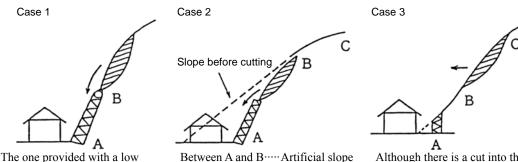
The one provided with a low masonry wall or the like only, and not cut into its slope, judging from the present topography, shall be deemed to be a natural slope.
