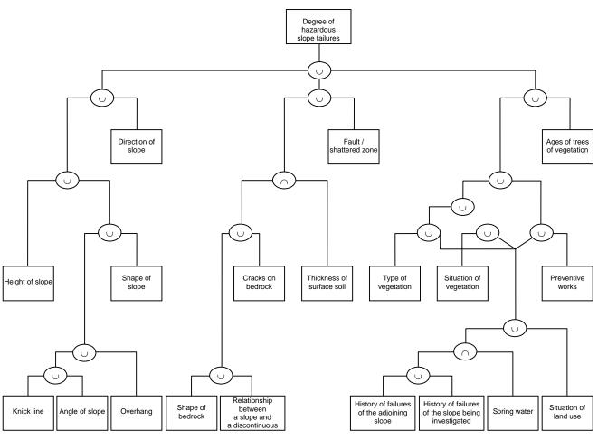
Fig-3 Structurization of slope failures at the time of rainfall
