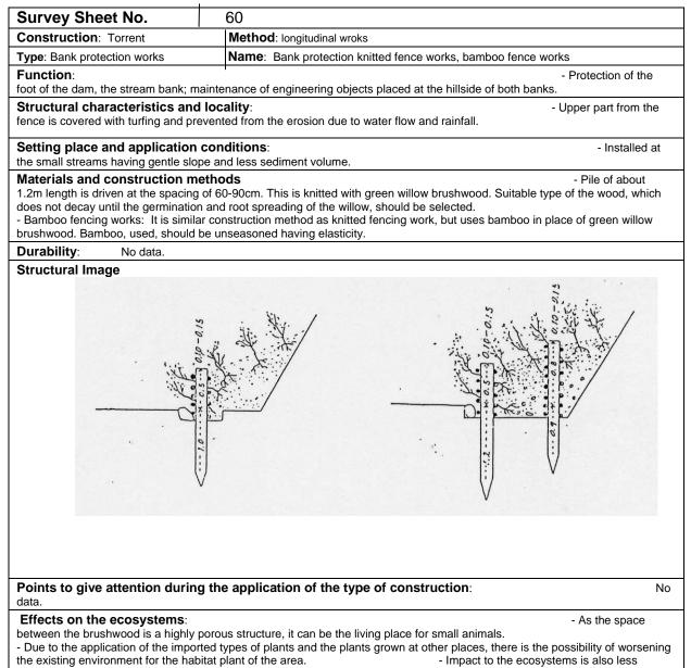
compared to the concrete structure.
