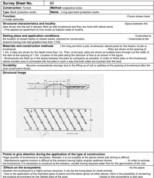
compared to the concrete structure.
