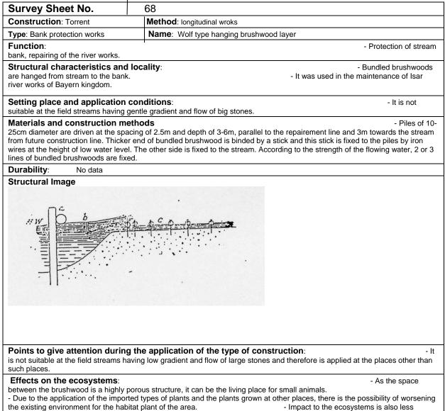
compared to the concrete structure.
