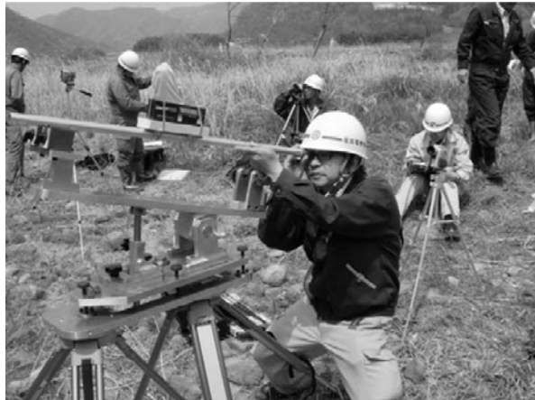
Photograph Appendix 6 Measurement using an angle gauge
