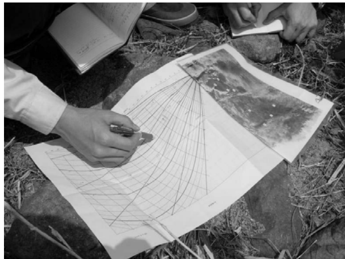
Photograph Appendix 8 Estimation of an elevation angle using a quick chart
