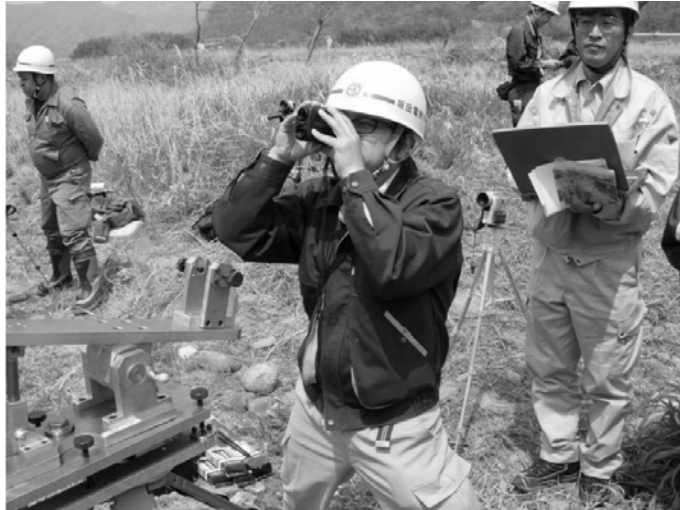
Photograph Appendix 7 Measurement of diagonal distance using a laser rangefinder
