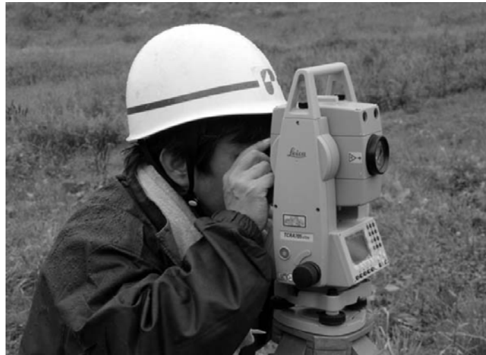
Photograph Appendix 9 Measurement using the total station
