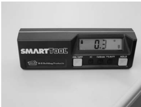
Photograph Appendix 5 Digital inclinometer
