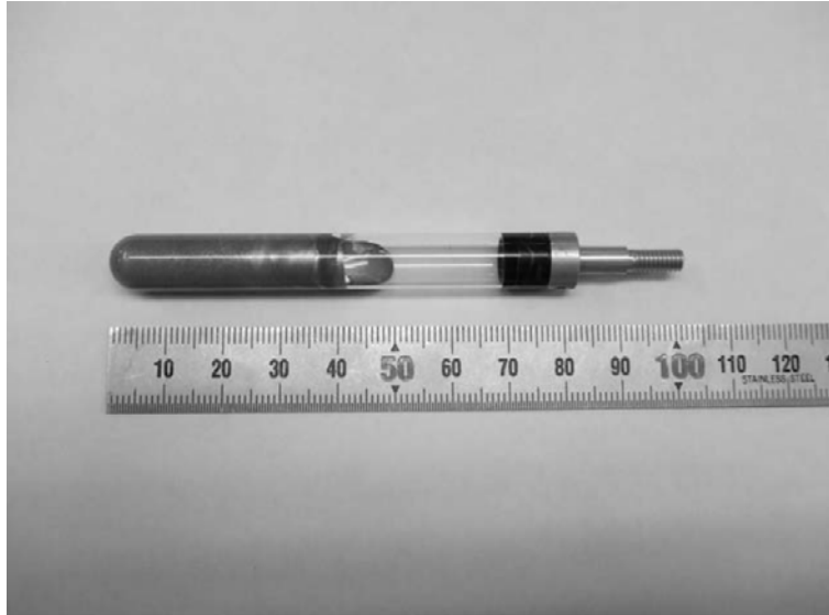
Photograph Appendix 2 Paint capsule
